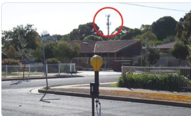
A survey site with the measurement device in the foreground and base station in the background
