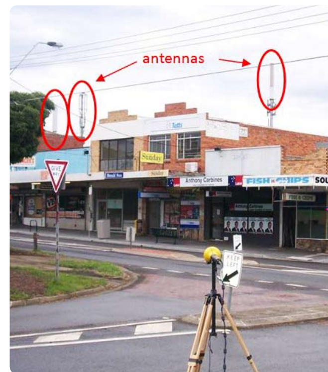
Radiofrequency levels at Heidelberg Heights were recorded at 0.265 per cent of the safety limit
