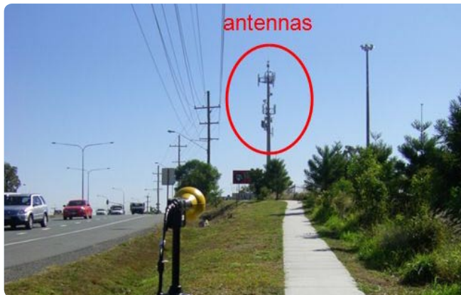
The maximum measurement recorded in Calamvale, QLD, was only 0.051% of the safety standard limit
